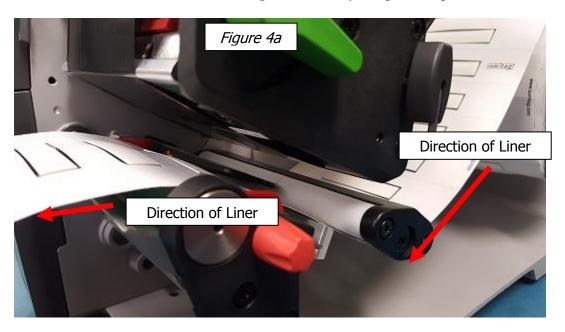
b. Using the red knob, adjust the red fingers until they are in close proximity, but not touching, the liner on each side.
